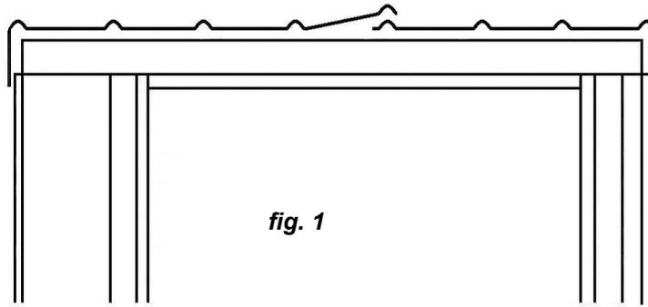
**Step 1: Note:** Condensation can form on the under side of shed roof. If building paper is required, fit now. Building paper will need to be supported by netting or roofing twine.
